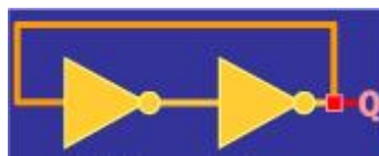
Fig.1: Simplest realization of feedback circuit
