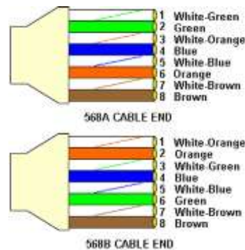
Figure 1.9: EIA/TIA 568A and 568B
