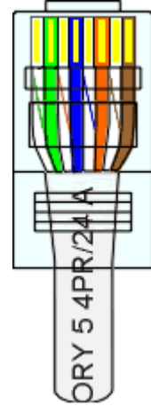
Figure 1.10: Preparing the RJ-45
