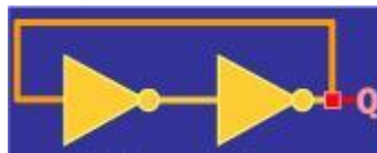
Fig.1: Simplest realization of feedback circuit
