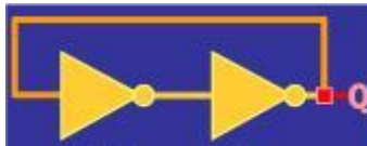
Fig.1: Simplest realization of feedback circuit
